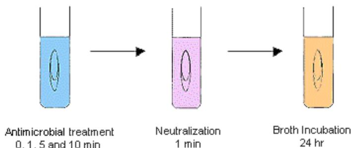
FIG. 1. Diagram showing the steps for Day one of the use dilution assay.
