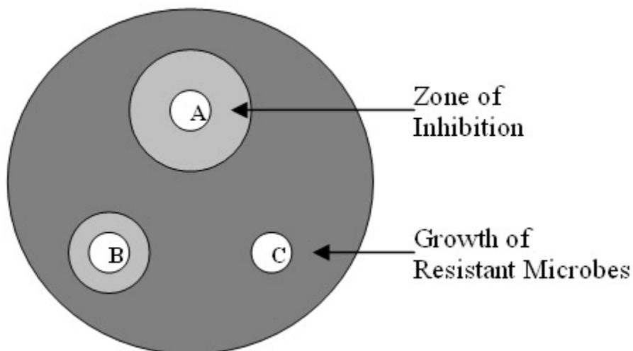
FIG. 1. Agar disc diffusion test for microbial sensitivity to antibiotics, disinfectants, antiseptics, or sanitizing agents. The chemical on disc A has a larger zone of inhibition than the chemical on disc B. The chemical on disc C has no inhibitory effect upon the growth of microbes, thus there is no zone of inhibition.
