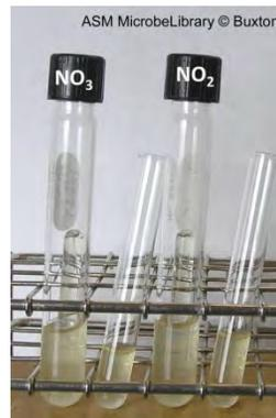
FIG. 15. Addition of reagents A and B to both the nitrate and nitrite broth results in no color change in either broth. These results indicate the reduction of the  $\text{NO}_2^-$ , but whether
