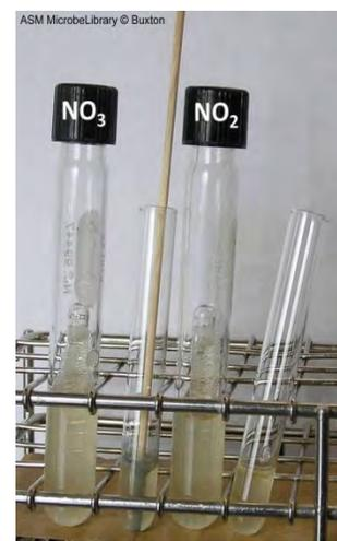
FIG. 13. Addition of zinc to the  $\text{NO}_3^-$  broth results in no color change. This result indicates reduction of  $\text{NO}_3^-$ .
