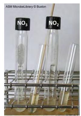
FIG. 17. Addition of zinc to the nitrate broth incubated for 48 hours results in no color change. This result indicates the complete reduction of  $\text{NO}_3^-$ .
