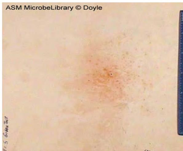
FIG. 2. Results of the modified Griess test for the shirt shown in Fig. 1.
