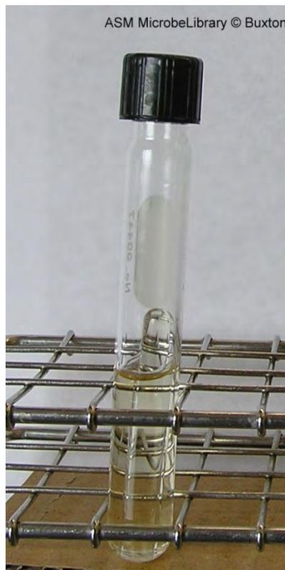
FIG. 3. The pressure of autoclaving forces broth into the Durham tube.
