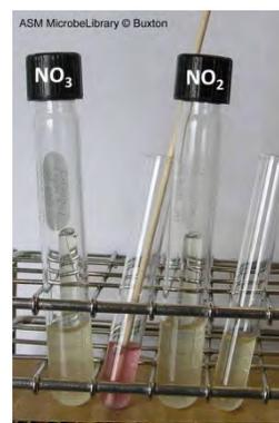
FIG. 16. Addition of zinc to the nitrate broth incubated for 24 hours results in a weak color. This result indicates partial reduction of  $\text{NO}_3^-$ .
